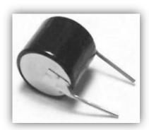
Other **CMOS** batteries include the barrel design (shown), also soldered into the board, and plug-in packs. They supply 3V and are typically rated to last 5 to 10 years.
