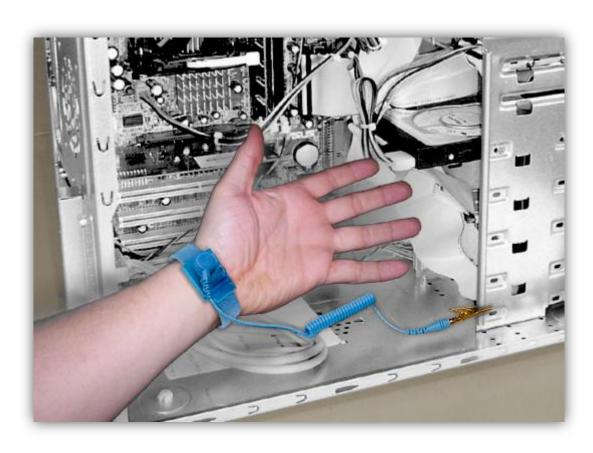
Antistatic wrist or ankle straps should <u>NEVER</u> be worn while working on higher voltage components, such as monitors and power-supply units.
